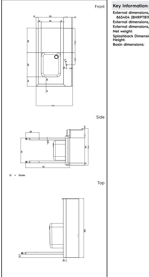
External dimensions, Width: 865404 (BHRPTB11R) 1200 mm External dimensions, Depth: 755 mm External dimensions, Height: 1170 mm 22 kg Splashback Dimensions, Height: 260 mm
